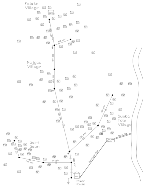
Figure 3: Electrical distribution network layout.
